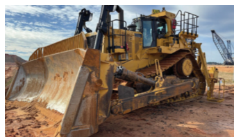
2018 CAT D11T - $1,588,000 1 owner, Cat Dealer preventative maintenance since new. Low hour components. UC measures like new, U Blade, MS ripper. Excellent condition.
