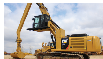
2018 CAT 336FL MH - $528,000 New J.J. Scheckel Material Handler Conversion pkg, 2,200 Hours, 54' Total reach, New 30' Boom, 24' Stick, Hydraulic lift cab, Cwt, Bucket or grapple available.
