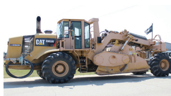
2009 CAT RM500 - $348,000 3,610 Hours, Reputation machine, Universal Rotor for both asphalt reclamation or soil mixing, Water emulsion system, Full service history.
