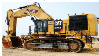
2021 CAT 6015B - $1,550,000 1,970 Total hours, 5 Year, 10,000 hour factory warranty until 2026. Mass Excavator Arrangement, 11'2" Stick, 24'9" Boom, 11.5 Yard 95" bucket, 1 Owner.
