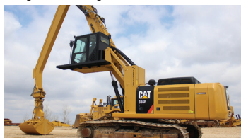
2018 CAT 336FL MH - $588,000 New J.J. Scheckel Material Handler Conversion pkg, 2,200 Hours, 54' Total reach, New 30' Boom, 24' Stick, Hydraulic lift cab, Cwt, Bucket or grapple available.
